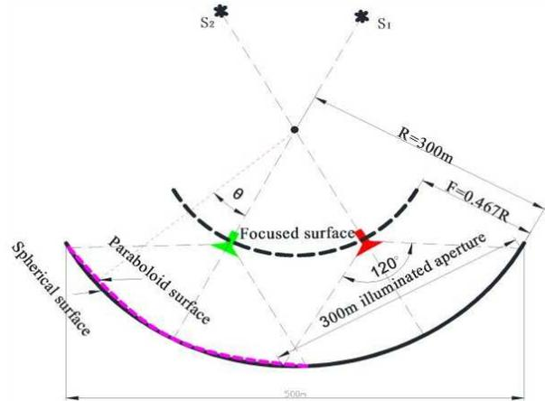
Fig. 2 Geometric optical principle of FAST.
