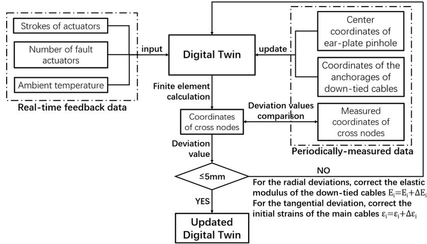
Fig. 4 The flow chart of updating process.
